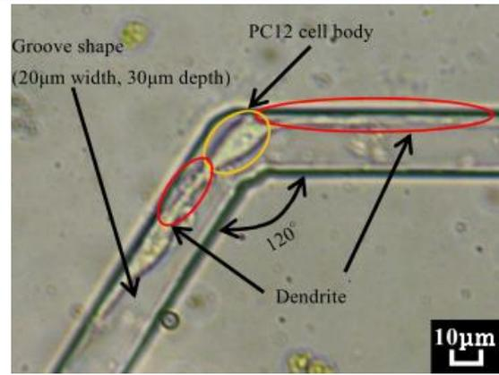
Fig. 4 Dendrite growth in 160 (upper) and 120° angled (lower) micro grooves
