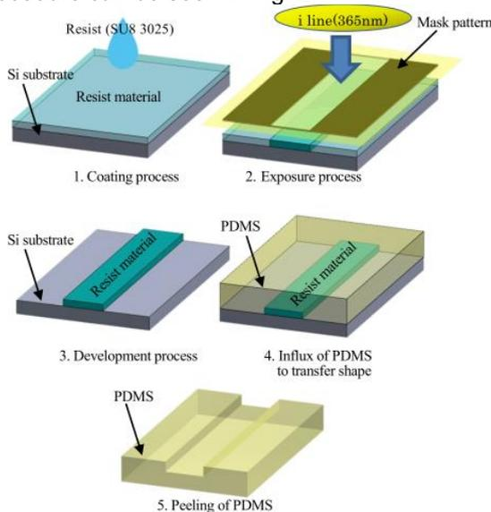
Fig. 2 Microfabrication process
