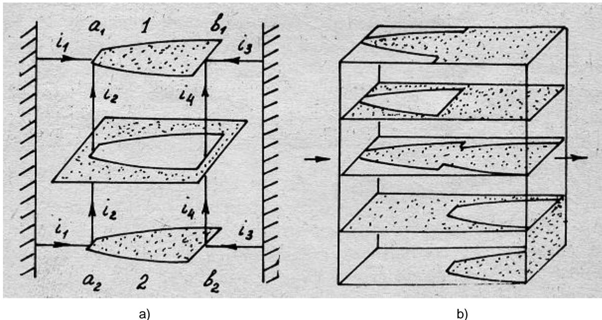
**Figure 1.** a) – balanced connection, which is implemented through the field diagram; b) – cascade connection of basic elements arranged in different layers of the multilayer package
