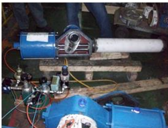
Fig.3 The torque measuring equipment Fig. 4 The cylinder motion with slider skew angle of 90 degrees
