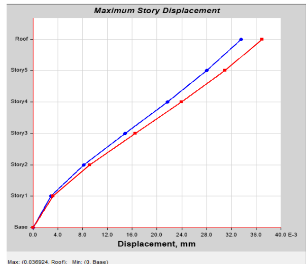
Fig. 5. Maximum Storey displacement (Etabs)
