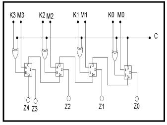
Figure (18) The logic design of the sub-function Z
