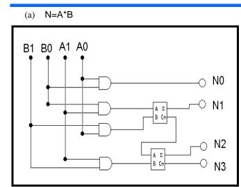
Figure (7) The logic design of the sub-function N
