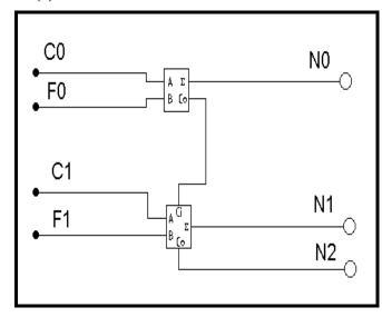
Figure (15) The logic design of the sub-function N (c) D=B+B
