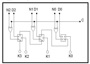
Figure (17) The logic design of the sub-function K
