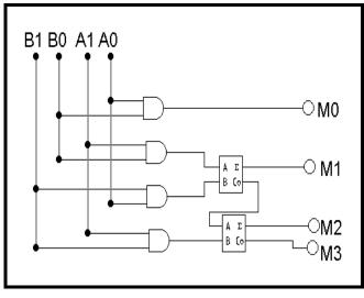
Figure (14) The logic design of the sub-function M
