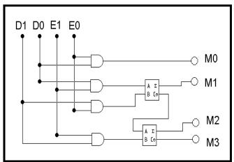
Figure (8) The logic design of the sub-function M (c) W=CF
