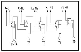
Figure (11) The logic design of the sub-function T (f) Z=T-W
