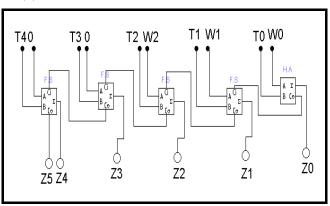
Figure (5) The logic design of the sub-function Z
