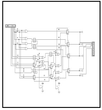
Figure (19) Implementation of third arithmetic unit ArU3
