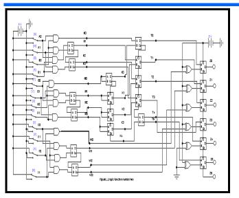
Figure (13) Implementation of second arithmetic unit ArU2
