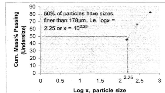
**Figure 6b: Cumulative Undersize Semilog Plot of Akwa Ibom**
