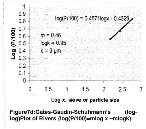
Figure 7d: Gates-Gaudin-Schuhmann's (log-log) Plot of Rivers { $\log(P/100) = m \log x - m \log k$ }
