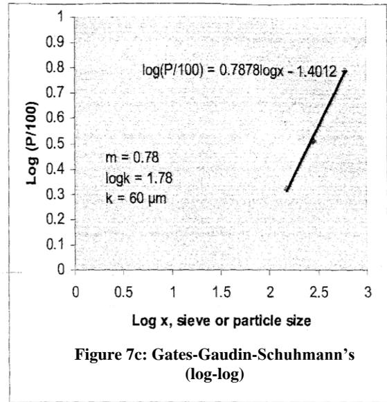
Figure 7c: Gates-Gaudin-Schuhmann's (log-log) Plot of Rivers { $\log(P/100) = m \log x - m \log k$ }
