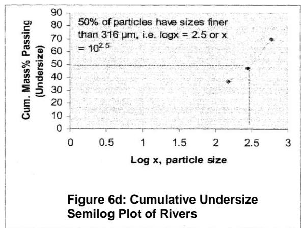
**Figure 6d: Cumulative Undersize Semilog Plot of Rivers**
