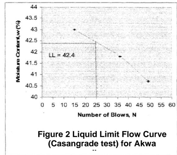
Figure 2: Liquid Limit Flow Curve (Casangrade test) for Akwa
