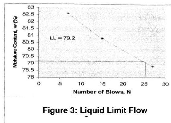
Figure 3: Liquid Limit Flow
