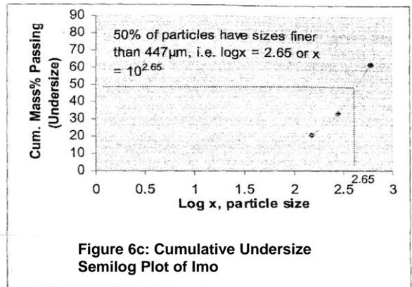
**Figure 6c: Cumulative Undersize Semilog Plot of Imo**
