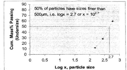
**Figure 6a Cumulative Undersize Semilog Plot of Abia**
