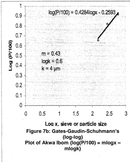
Figure 7b: Gates-Gaudin-Schuhmann's (log-log) Plot of Akwa Ibom { $\log(P/100) = m \log x - m \log k$ }
