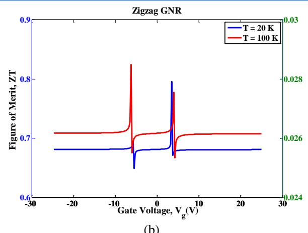
Fig.4. The variation of the figure of merit with gate voltage at different temperatures.
