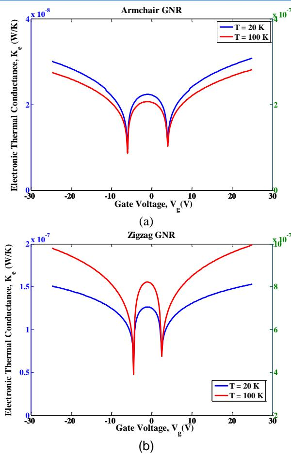
Fig.3. The variation of electronic thermal conductance with gate voltage at different temperatures.
