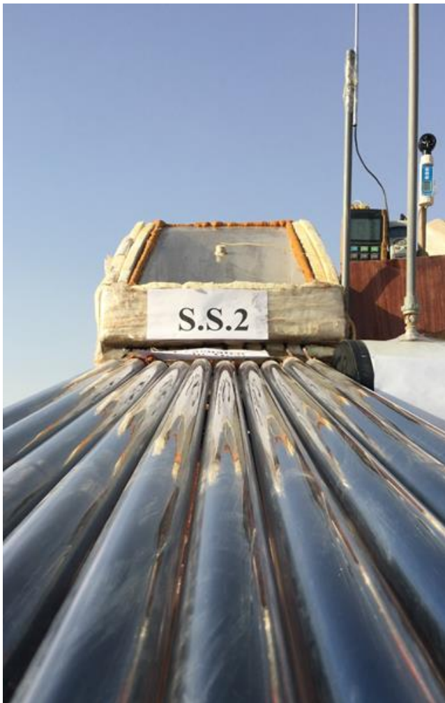
Figure 8. The evacuated tube heat pipes coupled with the still.
