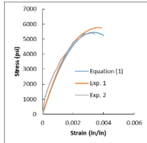
Fig. 1. Stress-strain relation of concrete
