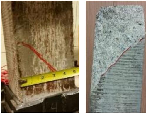
Fig. 10. Final crack pattern of SM01
