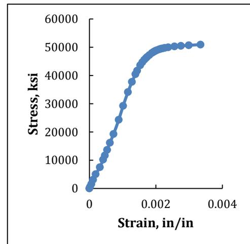
Fig. 2. Stress-strain relation of steel rebars
