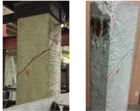
Fig. 13. Final crack pattern of SM02
