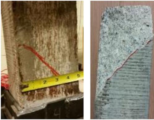
Fig. 10. Final crack pattern of SM01
