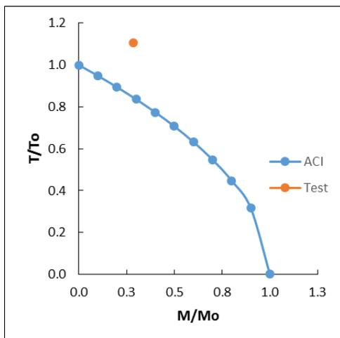
Fig. 19. Bending-torsion interaction for SM03
