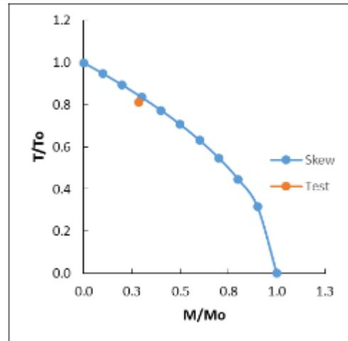
Fig. 20. Bending-torsion interaction for SM03
