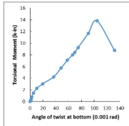
Fig. 15. Torsion versus angle of twist plot of SM03
