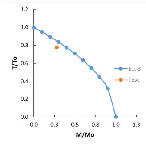
Fig. 18. Bending-torsion interaction for SM02
