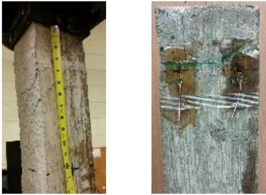
Fig. 16. Final crack pattern of SM03
