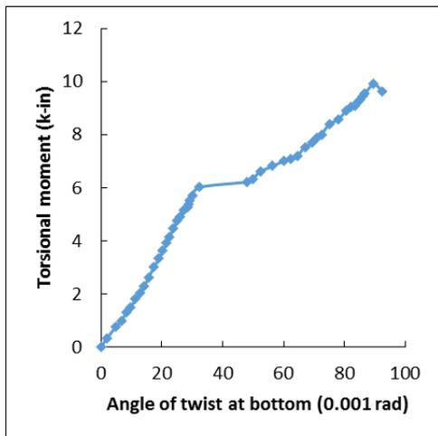
Fig. 12. Torsion versus angle of twist plot of SM02
