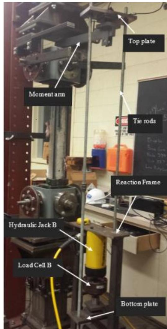
Fig. 6. Bending test setup
