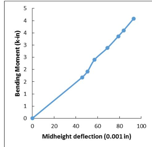
Fig. 8. Bending versus deflection plot of SM01
