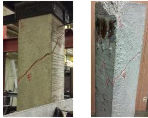
Fig. 13. Final crack pattern of SM02
