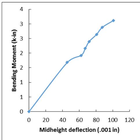
Fig. 11. Bending versus deflection plot of SM02
