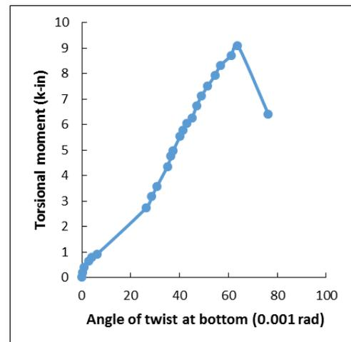
Fig. 9. Torsion versus angle of twist plot of SM01
