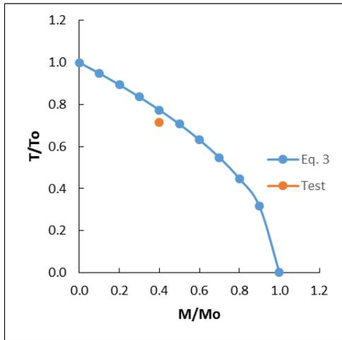
Fig. 17. Bending-torsion interaction for SM01
