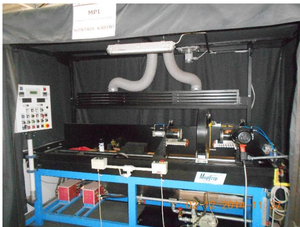
Fig. 8.. Magnetic particle inspection test bench
