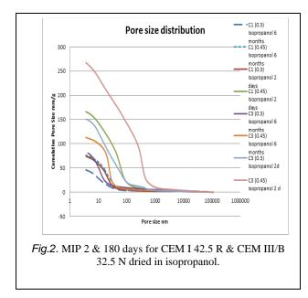
We see the same trend at the Figure 2, comparing system 4 cured for 2 and 180 days dried in isopropanol.
