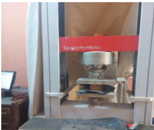
Fig. 1. Universal testing machine with compressive test cube
