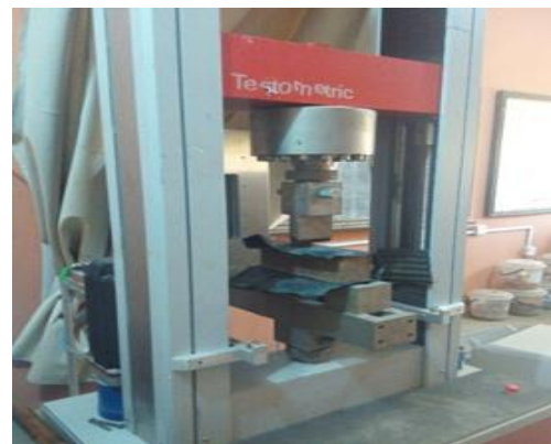
Fig. 3. UTM with flexural test sample
