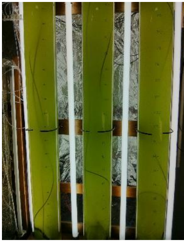
Fig. 3 Photobioreactors used to obtain biomass.
