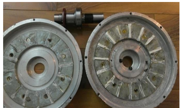
Fig-9 Rotor plates with the shaft and bearings
