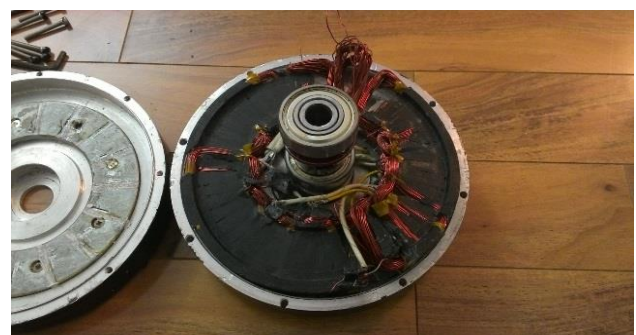
Fig-10 View of the coil and shaft
