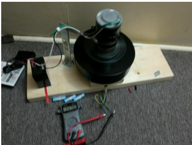
Fig 5 – Shows working of coreless generators being used currently in markets. With battery input and AC output in volts (147.5).
