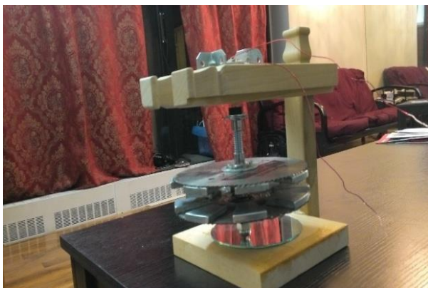
Fig 2 - Generator without stator coil
