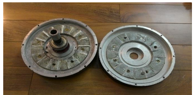
Fig-8 Internal view showing magnet slots on the rotor plates
