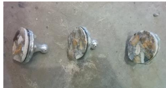
(b) Failed samples showing good bond.
