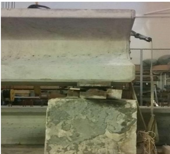
Fig. 10. Central load application, girder CF2.
