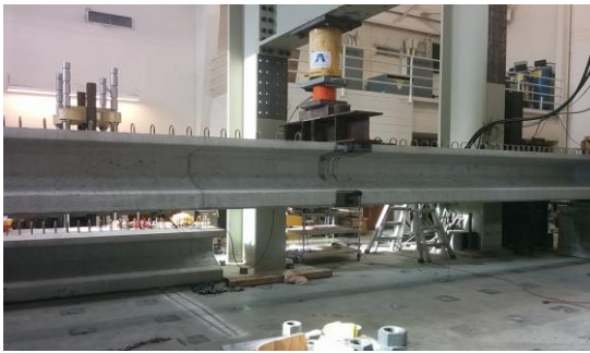
Fig. 10. Central load application, girder CF2.
