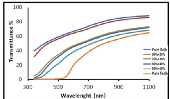
**Fig 1. The optical Transmittance of SnO<sub>2</sub>/ Fe<sub>2</sub>O<sub>3</sub> nanocomposite.**
