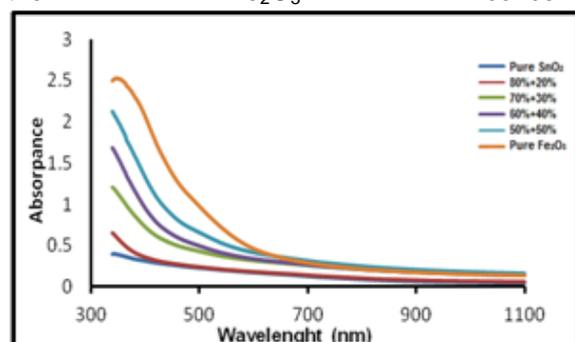
**Fig. 2. The optical Absorption of of SnO<sub>2</sub>/ Fe<sub>2</sub>O<sub>3</sub> nanocomposite .**
