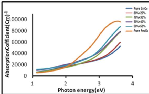
**Fig.3.**The absorption Coefficient of of SnO<sub>2</sub>/ Fe<sub>2</sub>O<sub>3</sub> nanocomposite.
