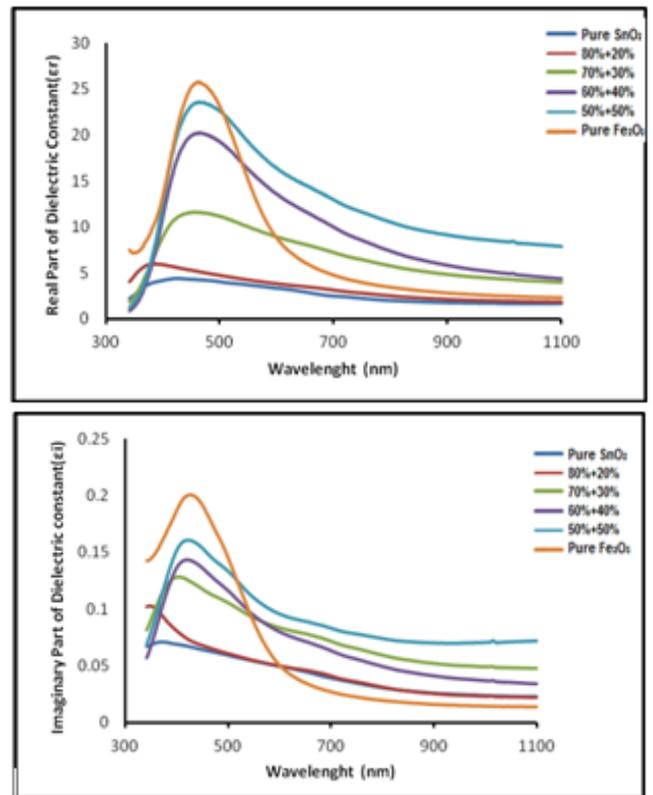
**Fig.9. The Real and Imaginary Parts of Dielectric Constant of SnO<sub>2</sub> /Fe<sub>2</sub>O<sub>3</sub> nanocomposite.**
