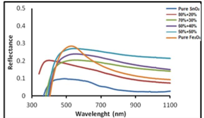
Fig.6 :The Reflectance of SnO<sub>2</sub> /Fe<sub>2</sub>O<sub>3</sub> nanocomposite.
