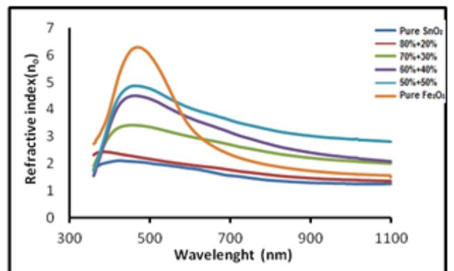
Fig.7.The Refractive index of SnO<sub>2</sub> /Fe<sub>2</sub>O<sub>3</sub> nanocomposite.
