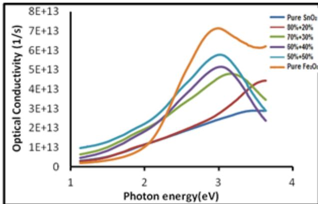
**Fig.10.The Optical Conductivity of SnO<sub>2</sub> thin films with different Fe<sub>2</sub>O<sub>3</sub> concentration.**
