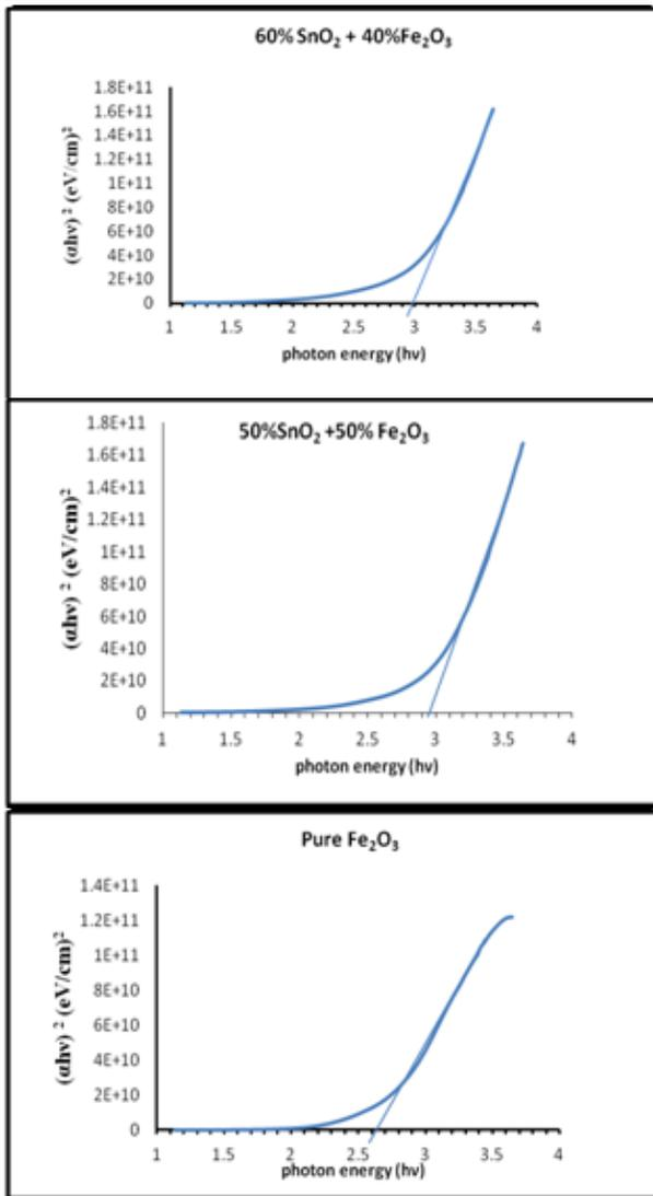
Fig.4. Variation of band gap for Fe<sub>2</sub>O<sub>3</sub>/ SnO<sub>2</sub> nanocomposite thin films prepared at different Fe<sub>2</sub>O<sub>3</sub> concentration.
