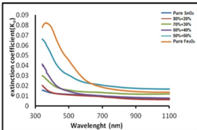
**Fig.8. The Extinction Coefficient of SnO<sub>2</sub> /Fe<sub>2</sub>O<sub>3</sub> nanocomposite.**
