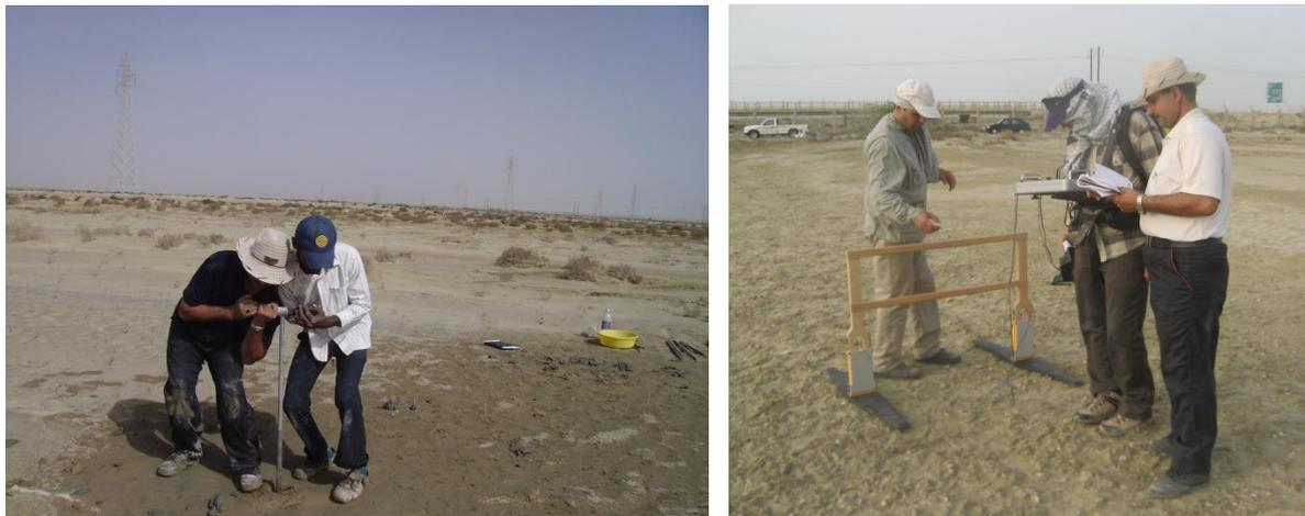
Fig. 2) The GPR device model Mala Geoscience-3 Step charger (right) and Core-consuming manual Auger (left).
