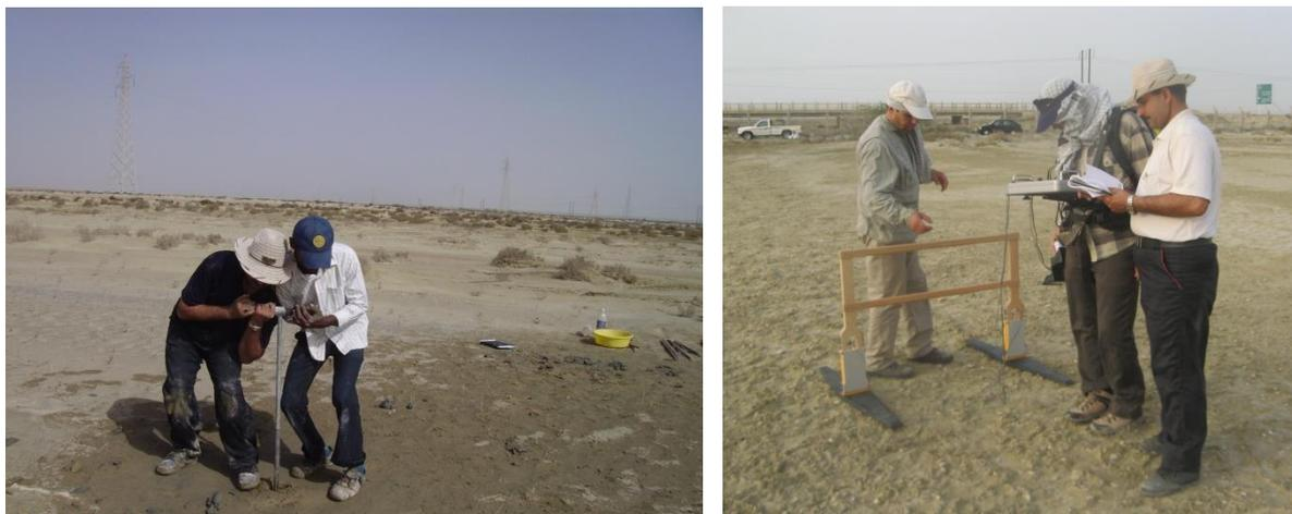
Fig. 2) The GPR device model Mala Geoscience-3 Step charger (right) and Core-consuming manual Auger (left).
