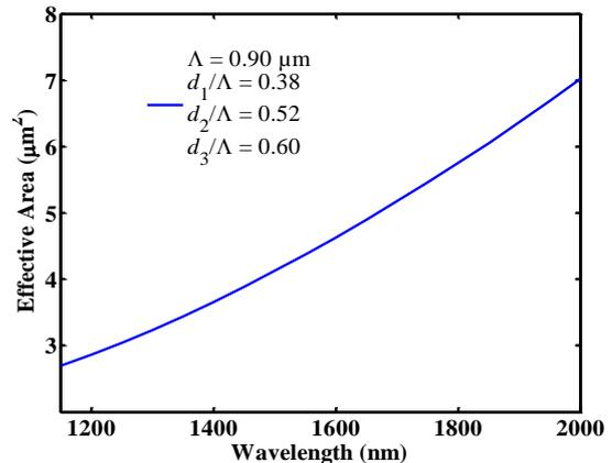
Fig. 7 Effective area Curve for optimum dispersion curve.
