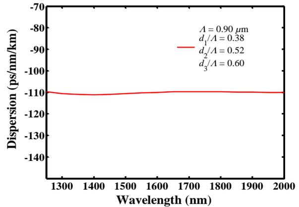
Fig. 2 Flattened negative dispersion at optimum design parameters.
