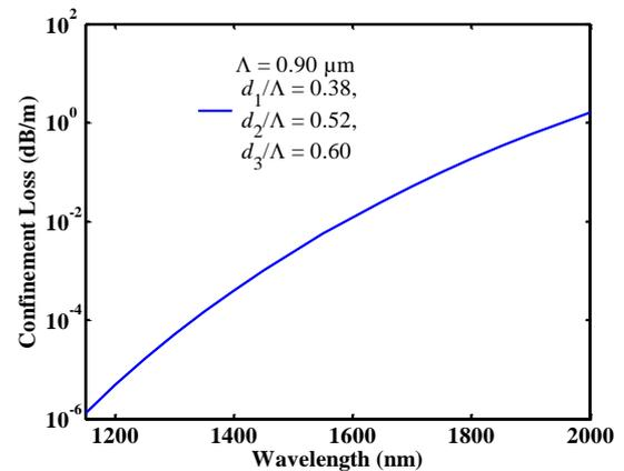
Fig. 8 Confinement loss curve for optimum dispersion parameter.
