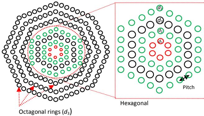
Fig. 1 (a) Cross-section of the proposed HyPCF, and (b) Illustration of the structure parameters.
