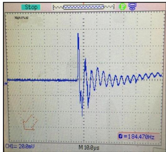
**Fig. 10. Images for Lifetime heterojunction MnS:Al/Si**
