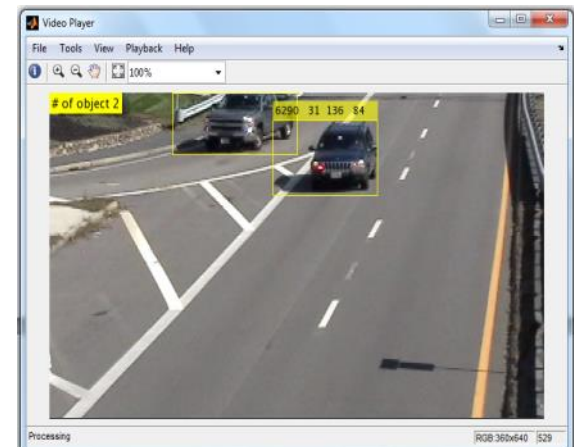
Fig. 4. c. shows the two detected objects ( two cars)
