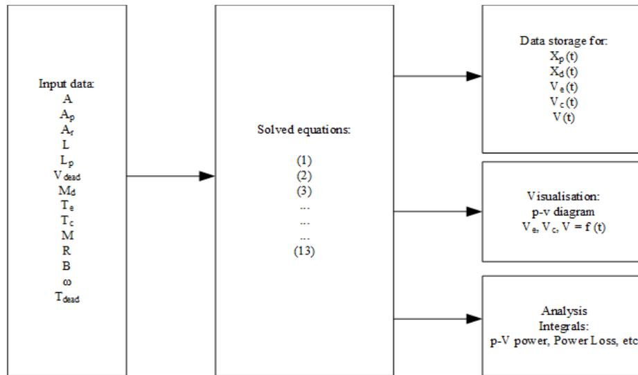
Fig. 5. The principle structure of TUS-SRSim computational procedure
