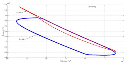
Fig. 11. *p-V diagrams of the investigated hybrid Stirling-Ringbom engine working with the design working fluid mass under different ambient pressures*
