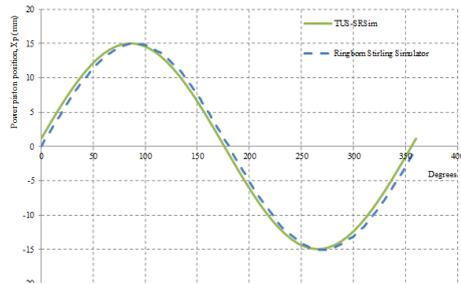
Fig. 7. *Time variation of the power piston position*
