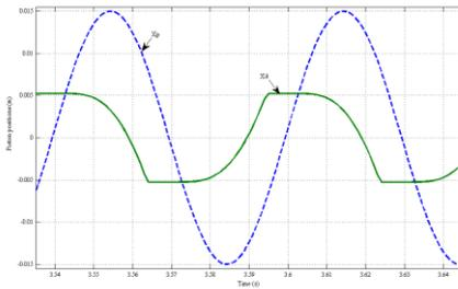
Fig. 9. *Time variation of the power piston  $X_p$  and the displacer  $X_d$*
