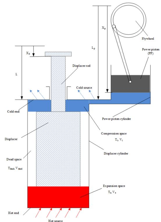
Fig. 2. Schematic diagram of the Stirling- Ringbom engine
