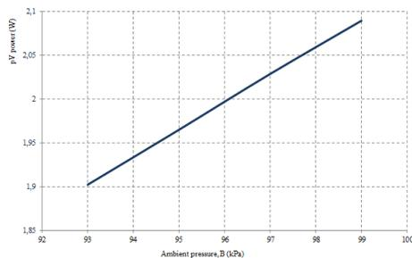
Fig. 14. *Cycle net power variation with the ambient pressure*
