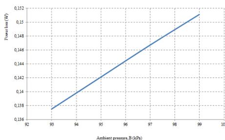
Fig. 15. *Variation of power loss with the ambient pressure*
