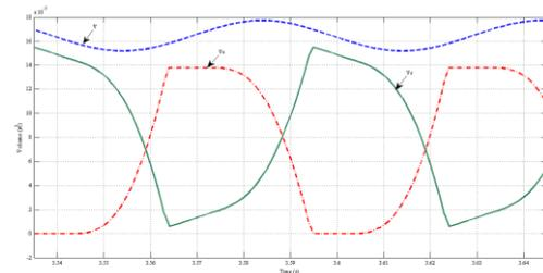
Fig. 10. *Time variation of the expansion volume  $V_e$ , compression volume  $V_c$  and the total volume  $V$*
