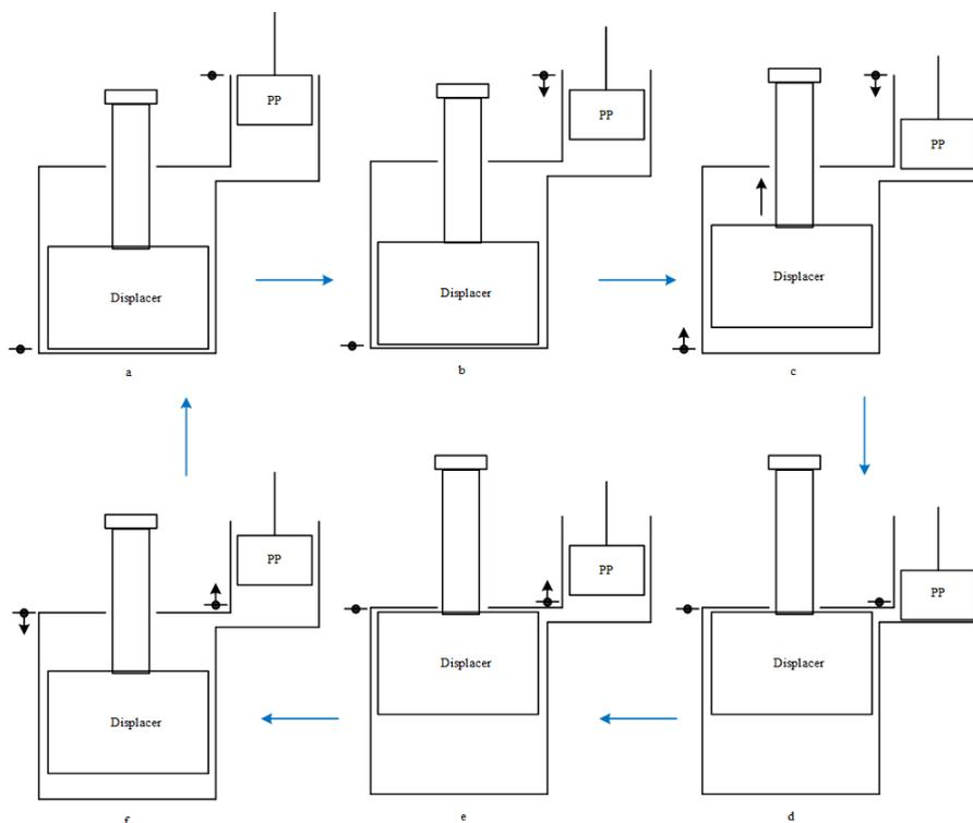
Fig. 3. Sequence of events for one cycle of Stirling-Ringbom engine
