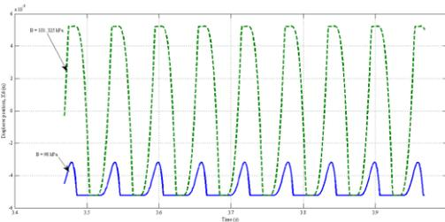
Fig. 13. *Displacer piston motion under design conditions and at ambient pressure of 98 kPa*
