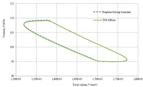
Fig. 6. *p-V diagrams of the simulated Stirling-Ringbom engine*
