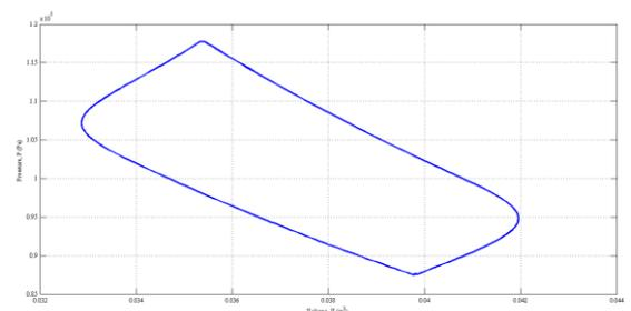
Fig. 4. p-V diagram of a hybrid Stirling-Ringbom engine cycle, [8]
