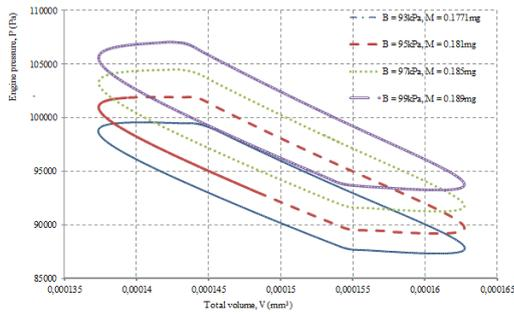
Fig. 12. *p-V diagrams of the Stirling-Ringbom engine at varying ambient pressure B and the corresponding working fluid mass M*
