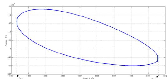
Fig. 1. p-V diagram of the Stirling engine with kinematically linked pistons, [8]
