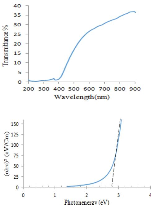
**Fig.3: Transmittance Spectra of CdO thin film and  $(\alpha h\nu)^2$  versus photon energy gap of CdO thin film continuously**
