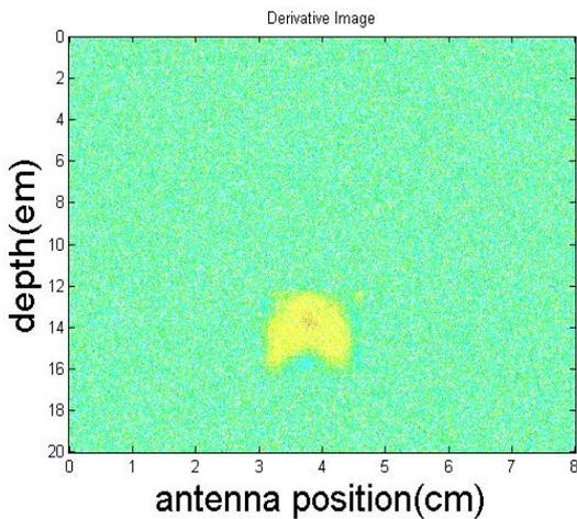
Fig. 8. Image of the absolute value of  $s_{cdern,m}$ . The reflections of a plastic mine buried in sand are noticeable.
