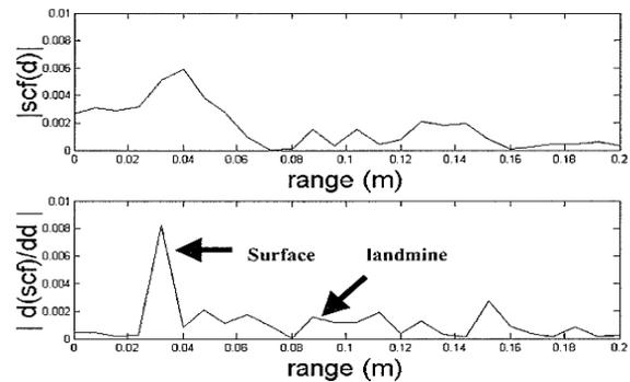
Fig. 5. scf range profile(top), sder range profile (button)
