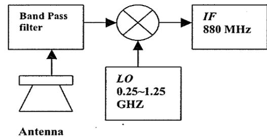
Fig .2. Block diagram of the GPR receiver
