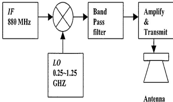
Fig .1. Block diagram of the GPR transmitter
