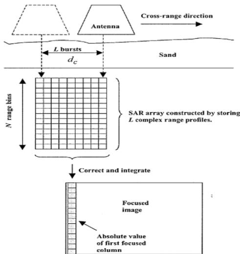
Fig. 6. SAR image being formed
