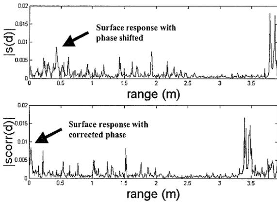
Fig. 3. (Top) sampled signal range profile, (Bottom) corrected signal range profile generated for a buried plastic landmine in sand
