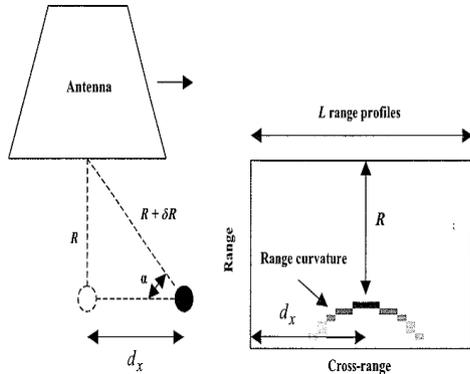
Fig. 7. GPR moving and an example of unfocused image obtained by displaying the absolute value of the SAR array.
