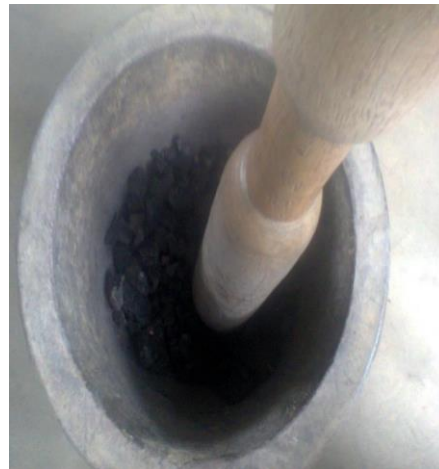
Fig. 5: Grinding the dry Chikoko soil
