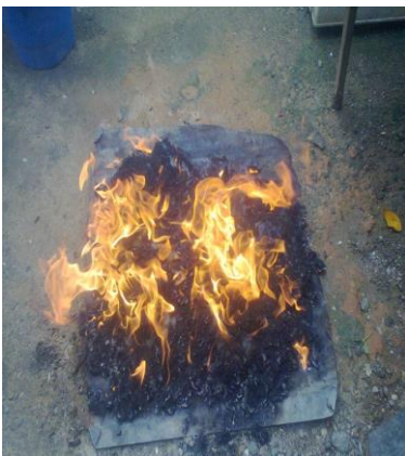
Fig. 2: Picture showing burning of the palm oil fibre
