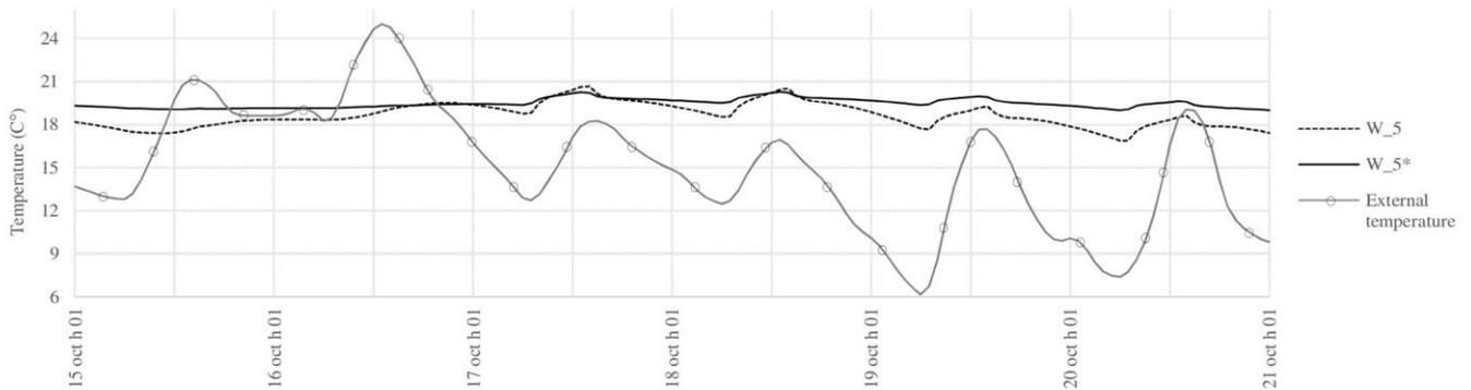
Fig. 11. Comparison between superficial temperatures of  $W_5$  and  $W_5^*$  in relation to outdoor highest temperatures from October the 15th to October the 21st.
