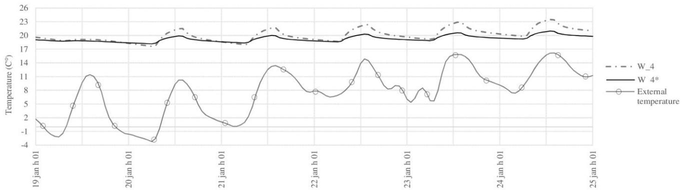
Fig. 10. Comparison between superficial temperatures of  $W_4$  and  $W_4^*$  in relation to outdoor lowest temperatures from January the 19th to January the 25th.
