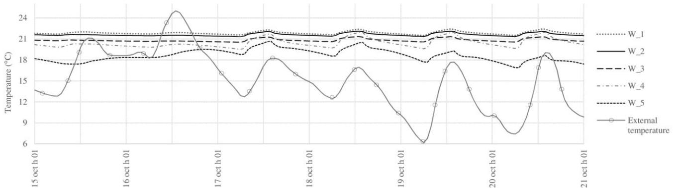
Fig.7. Comparison between the indoor superficial temperatures of the five walls with the highest outdoor temperatures from October the 15<sup>th</sup> to October the 21<sup>st</sup>.
