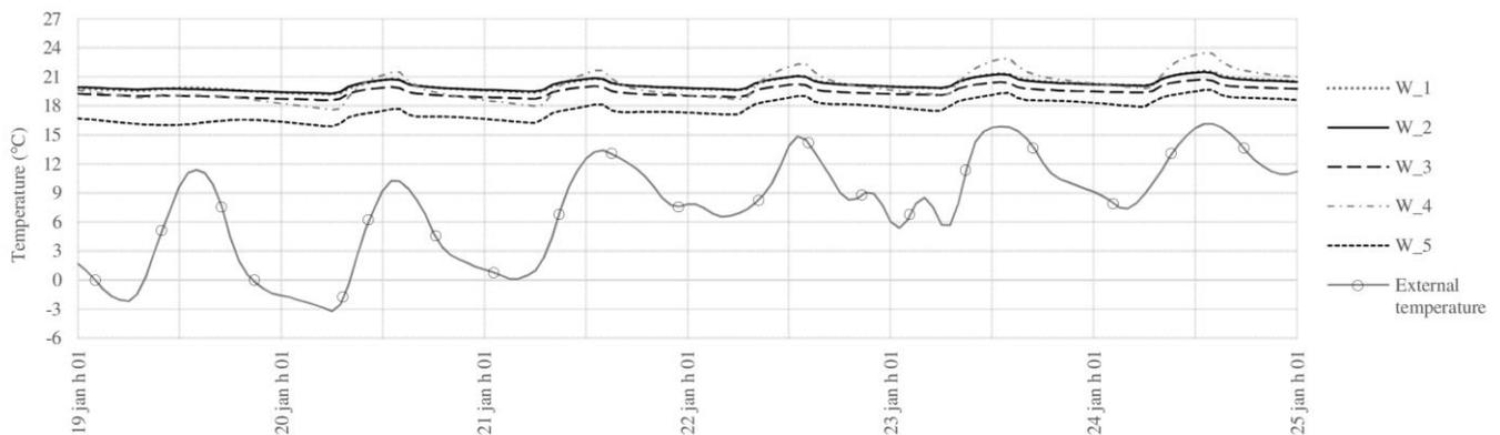
Fig. 8. Comparison between the indoor superficial temperatures of the five walls with the lowest outdoor temperatures from January the 19<sup>th</sup> to January the 25<sup>th</sup>.
