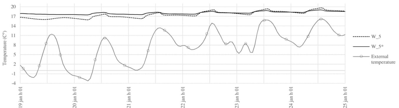
Fig. 12. Comparison between superficial temperatures of  $W_5$  and  $W_5^*$  in relation to outdoor lowest temperatures from January the 19th to January the 25th.
