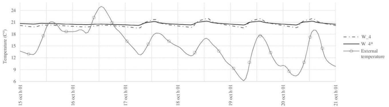
Fig. 9. Comparison between superficial temperatures of  $W_4$  and  $W_4^*$  in relation to outdoor highest temperatures from October the 15th to October the 21st.
