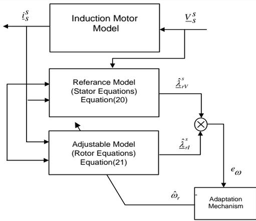
Fig.1: Basic configuration of saturated MRAS speed estimation
