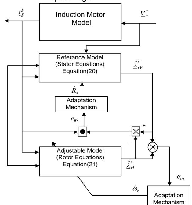
Fig.2: Structure of saturated MRAS system for parallel rotor speed and stator resistance estimation.
