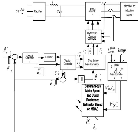
Fig.3: Block diagram of the proposed sensorless indirect vector controlled induction motor
