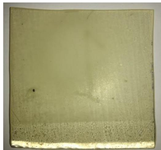
Fig.3 unfiled with oil epoxy specimen
