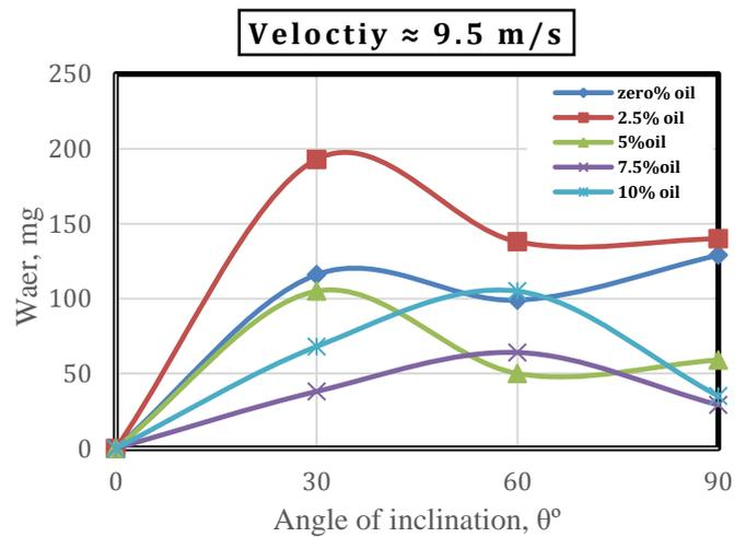
Fig.6 Relationship between impact angle and weight loss for 60 mm distance far from sand jet
