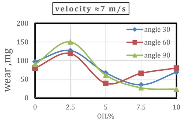
Fig.10 Relationship between oil content and wear at 7 m/s particle velocity.
