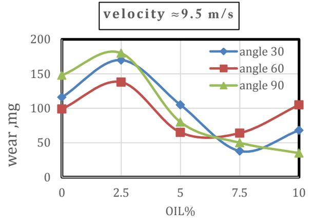
Fig.9 Relationship between oil content and wear at 9.5 m/s particle velocity.
