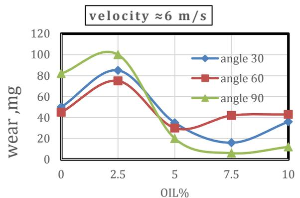
Fig. 11 Relationship between oil content and wear at 6.5 m/s particle velocity.
