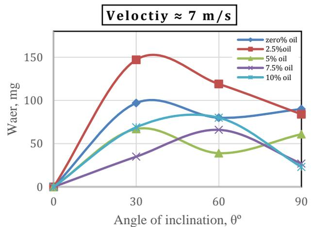
Fig. 7 Relationship between impact angle and weight loss for distance 100 mm far from jet.
