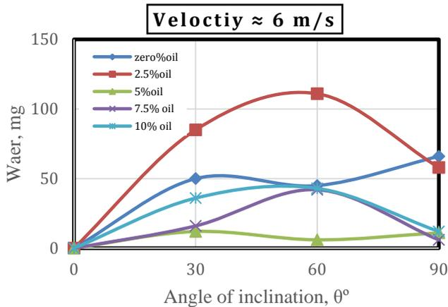
Fig.8 Relationship between impact angle and weight loss for distance 160 mm far from sand jet.
