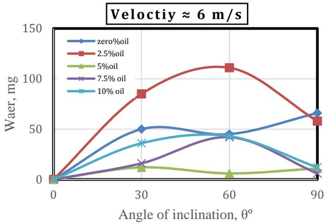
Fig.8 Relationship between impact angle and weight loss for distance 160 mm far from sand jet.
