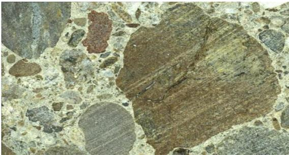
Figure 9: Standard Sample of concrete at 400<sup>0</sup>C
