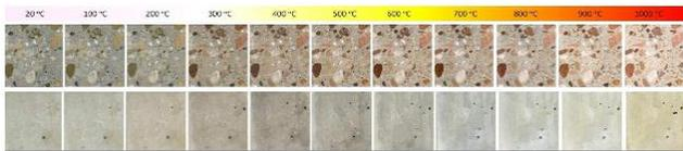
Fig 1: Color change of heated concrete: surface with exposed aggregates and external surface of the concrete specimen
