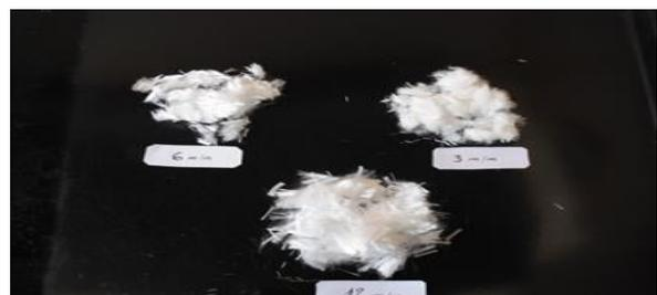
Figure 3 : Polypropylene fiber of length 3mm, 6mm and 12 mm.
