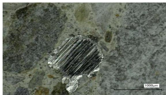
Figure 14 : Steel Sample of concrete at 200<sup>0</sup> C
