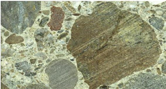
Figure 9: Standard Sample of concrete at 400<sup>0</sup>C
