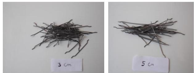
Figure 2 : Steel Fiber of length 3 cm and 5 cm
