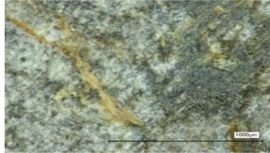
Figure 11 : Polypropylene Sample of concrete at 200<sup>0</sup>C
