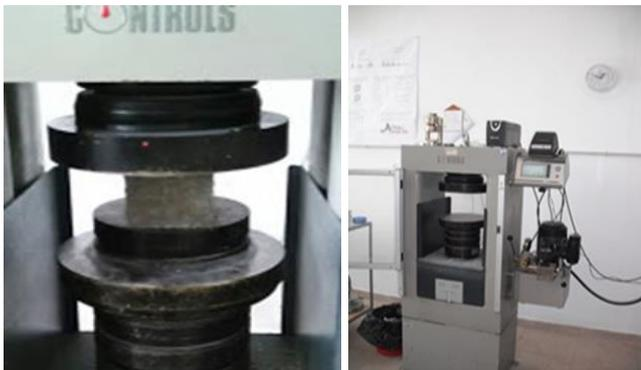
Figure 5 .Compressive strength test on compressive test machine
