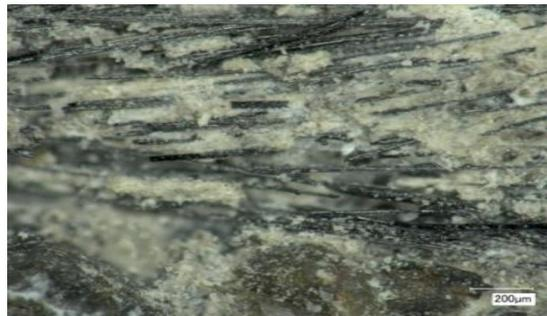
Figure 12 : Polypropylene sample of concrete at 400<sup>0</sup>C
