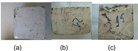
Figure 6: Samples after heat exposure at (a) 200°C, (b) 400°C and (c) 600°C
