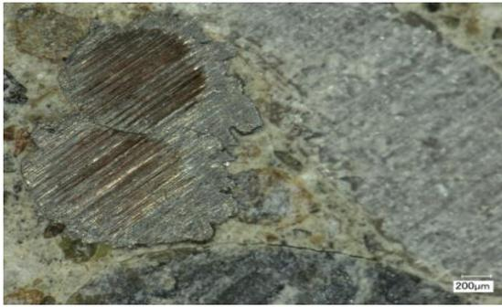
Figure 15 : Steel Sample of concrete at 400 °C
