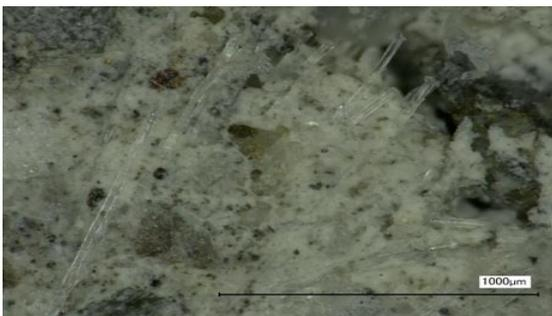
Figure10 : Polypropylene Sample of concrete at room temperature
