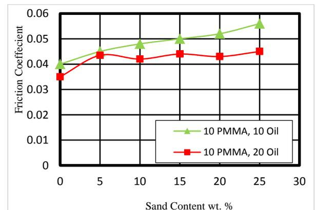
Figure 12 Friction coefficient of specimens after adding 0.4 wt. % graphene and different contents of sand content.
