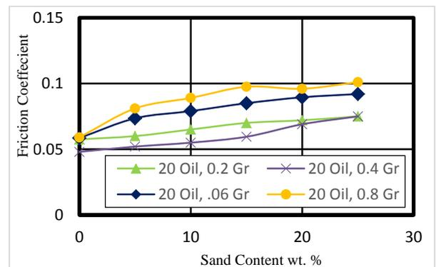
Figure 6 Friction coefficient of specimens with grease different contents of nano graphene and sand.
