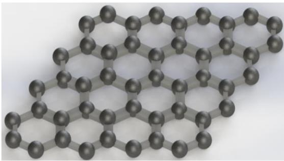
Figure 8 Graphene layer.
