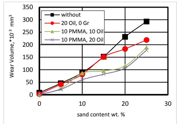
Figure 11 Relation between sand content and wear with different contents of PMMA and oil.
