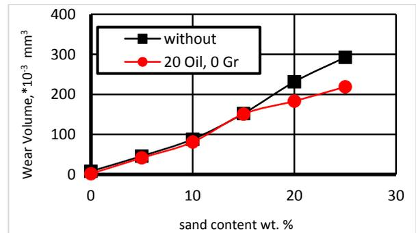
Figure 5 Wear volume of specimens Caused by abrasive sand particles.
