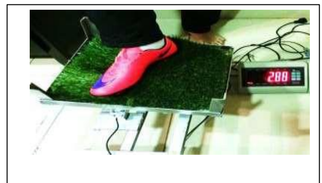
Fig.3 Application of the load.
