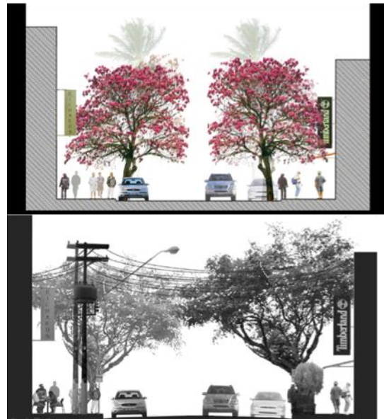
Figure 6. Comparison between the situation with utility poles and overhead wiring (before the project) and the situation with underground system of networks and cable (after the project) Source: Vigliecca & Associates
