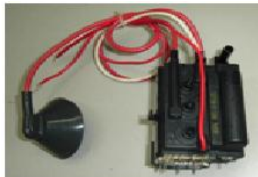
Figure 1.2: A typical TV flyback transformer
