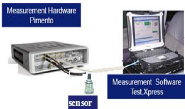
Figure 4: Typical setup of transducer-data acquisition pair
