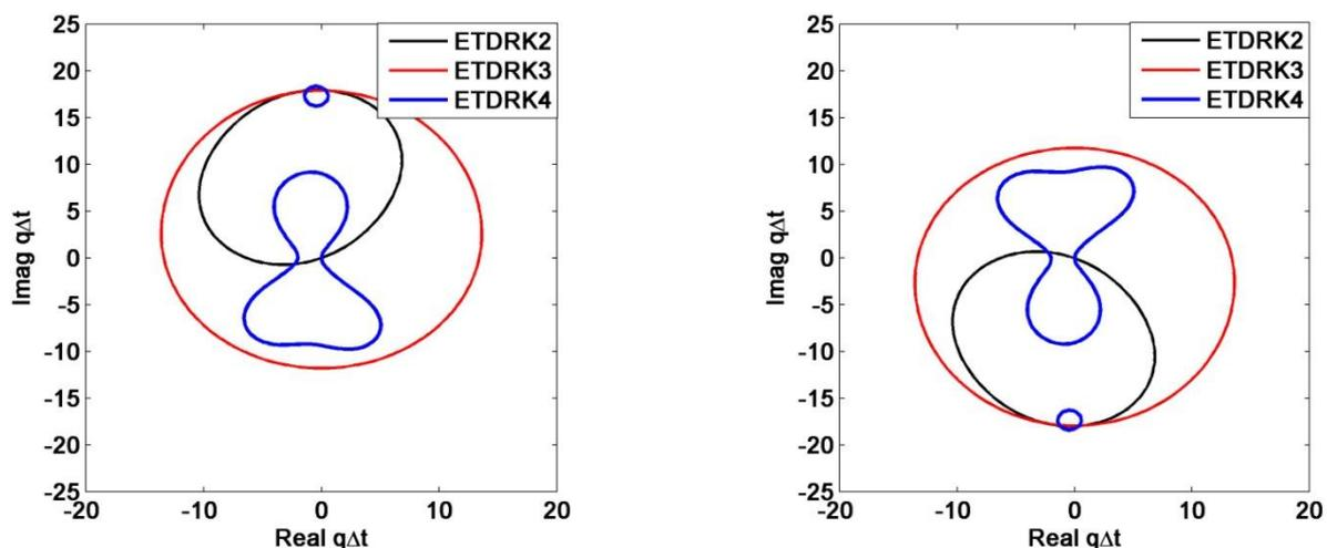
Fig. 2. Boundary of stability regions :ETDRK2, ETDRK3, ETDRK4 (a)  $y=-18i$ , (b)  $y=18i$
