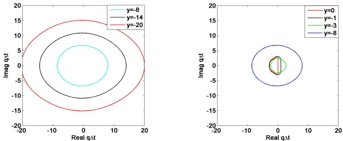
Fig. 1. Stability regions for RK4 and ETRK4 schemes in the complex plane of  $x=qt$  for several negative  $y=pt$
