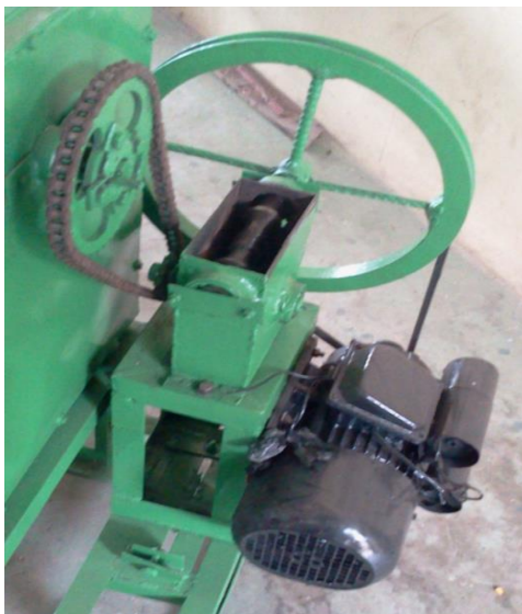
Plate 1.2 Arrangement of electric motor, gear box and paddle/stirrer shaft.
