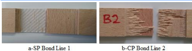
Figure 11. Failure types (a- Type 1, b- Type 2) of shear strength test.
