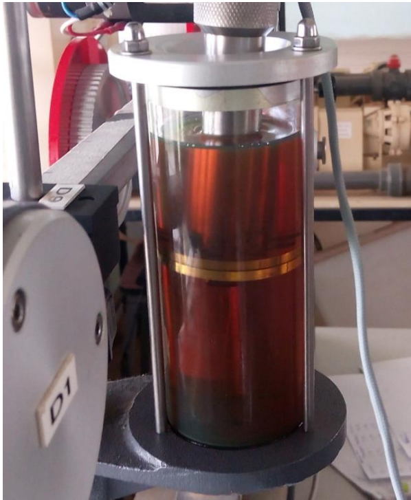
Figure: 3 Dashpot filled with oil sample
