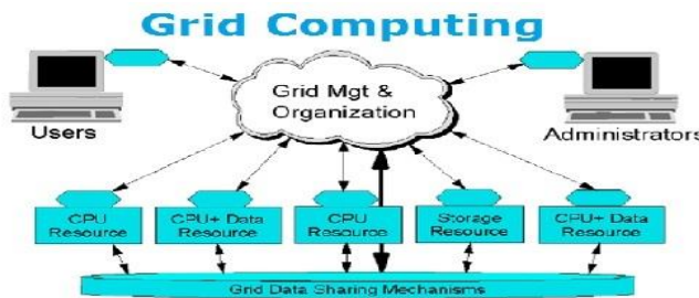
Figure 6: The diagram of grid computing infrastructure
