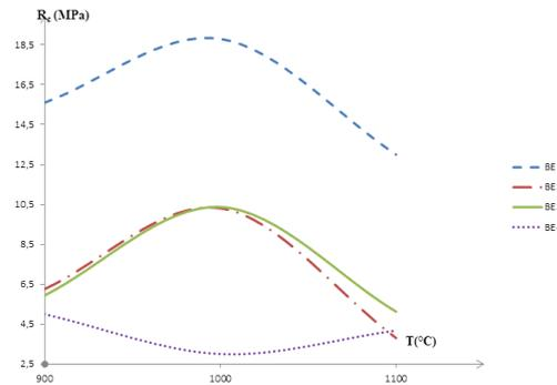
Figure. 6. Variation of compressive strength with the temperature
