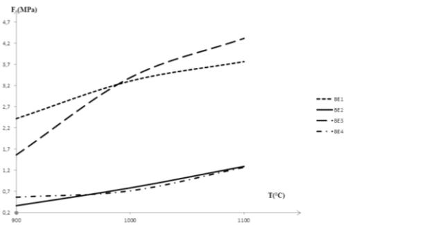
Figure. 7. Variation of flexural strength with the temperature
