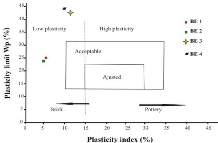
Figure. 4. Bain & Highley Diagram (1979) showing the position of our sample
