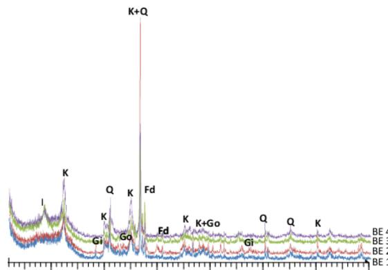
Figure 3. X-ray diffraction pattern (Cu K $\alpha_{1,2}$ ) of randomly non-oriented bulk sample showing the composition of sample analysis: I: illite; K: kaolinite; Gi: gibbsite; Go: goethite; Q: quartz; Fd: feldspath
