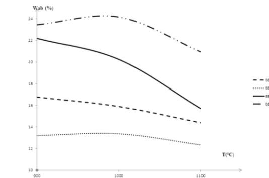
Figure. 8. Variation of water absorption with the temperature
