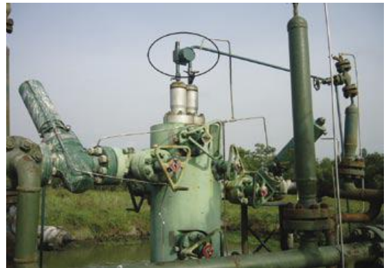
Fig.3. A vMbusX-SP wireless sensor units installed in an oil well in the Niger Delta by Shell to help prevent theft and sabotage [7]
