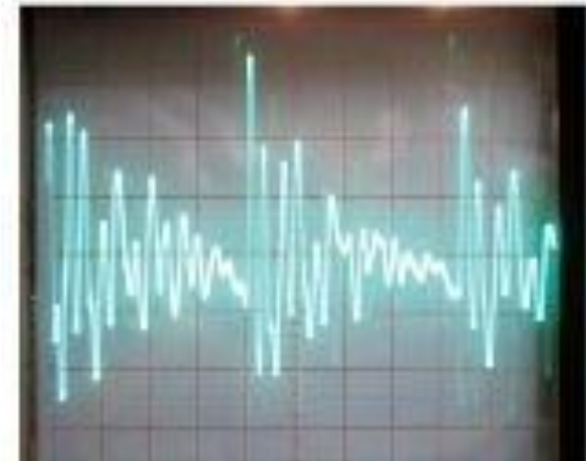
(b) Input signal of A/D converter which is output of microphone.
