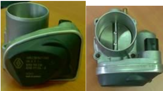
Fig. 1. Typical throttle body used in Internal Combustion Engine
