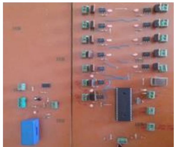
Figure 5. Microcontroller, USB and sensor card
