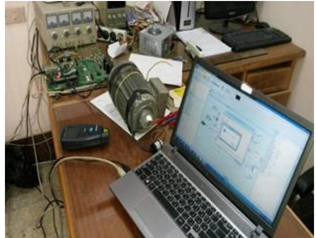
Fig. 28: Connection between MCB-2 Kit and Laptop using mZdsp 2812 Kit and XDS 100V2 emulator
