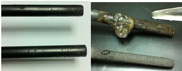
Fig. 4. Photo image of the graphite electrodes (A) before and (B) after static scale deposition and confirmation test with HCl.
