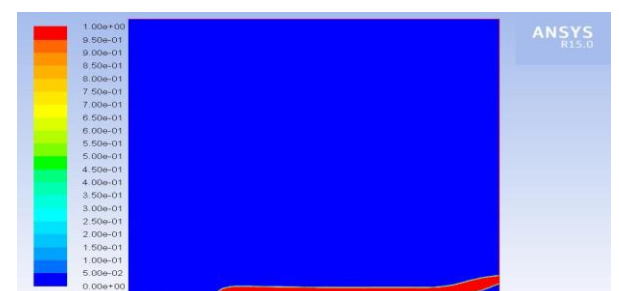
Fig. 7. Oil leak (60000 bpd, 1 m/s current velocity)
