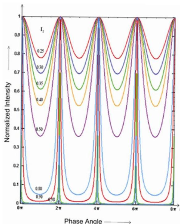
Fig.3: Intensity contour of Fringes due to multiple reflections
