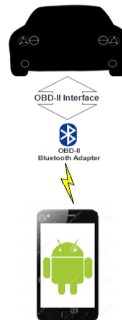
Fig. 1. Android-based OBD-II System
