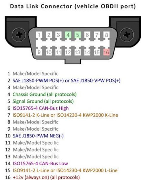
Fig. 2. Data Link Connector (SAE J1962) (Source: [6])
