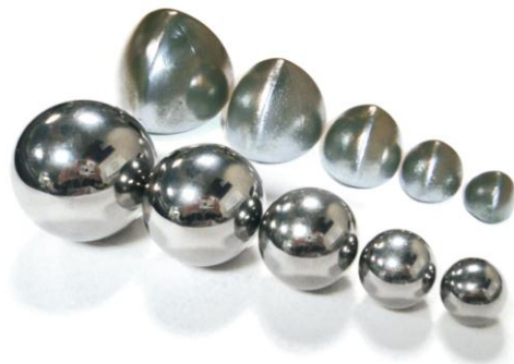
Fig. 3. Comparison of the two types of grinding bodies in the amount of 5 - spherical model and Relo body-M1.1, used in the tests of the Bond Mill.
