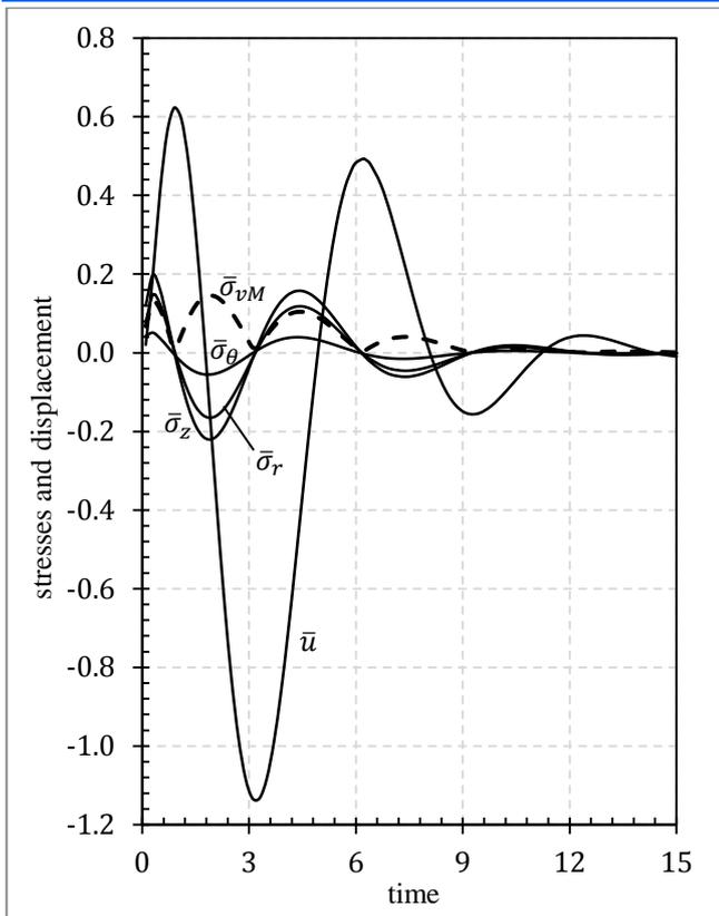
Fig. 3b. Variations of the stress components, the von Mises stress and the displacement with time at  $\bar{r} = 0.5$  based on B.C. 2 for the parameter set  $\nu = 0.3$ ,  $A = 2.0$  and  $\bar{\alpha} = 1.75$ .
