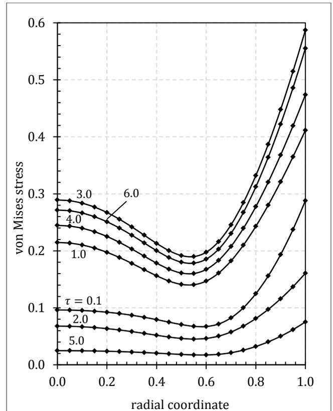
Fig. 1a. Distributions of the von Mises stress in the cylinder at various time instants based on B.C.1 for the parameter set  $\nu = 0.3$ ,  $A = 2.0$  and  $\bar{\alpha} = 1.75$ . The solid lines belong to the results of this work and dots to the numerical solution [16].
