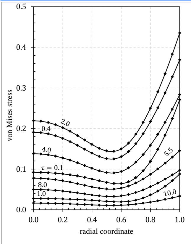
Fig.1b. Distributions of the von Mises stress in the cylinder at various time instants based on B.C.2 for the parameter  $\nu = 0.3$ ,  $A = 2.0$  and  $\bar{\alpha} = 1.75$ . The solid lines belong to the results of this work and dots to the numerical solution [16].
