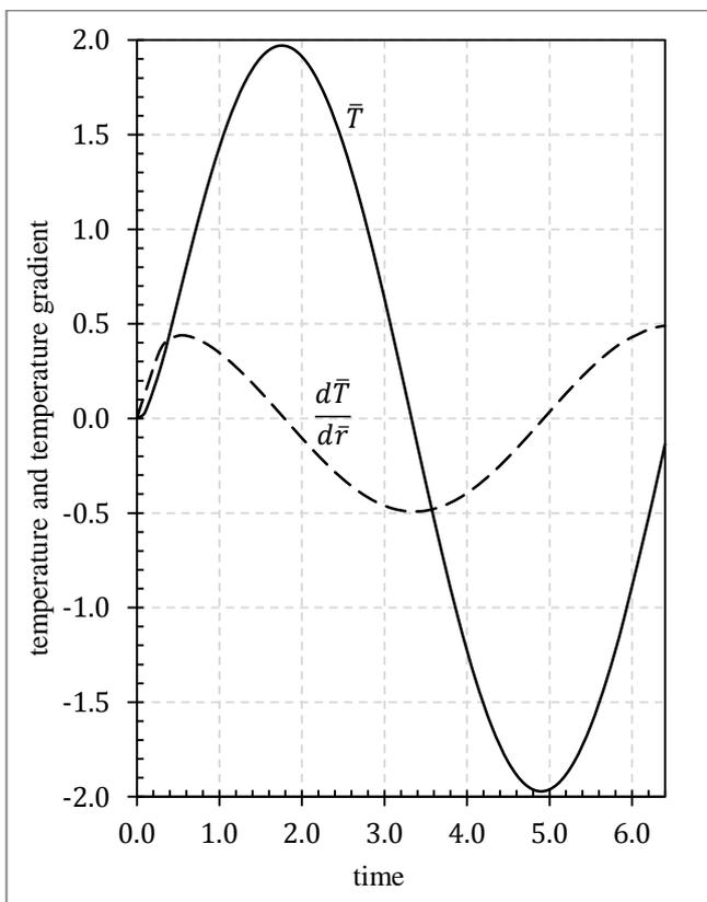
Fig. 2a. Variations of temperature and temperature gradient with time at  $\bar{r} = 0.5$  based on B.C.1 for the parameter set  $\nu = 0.3$ ,  $A = 2.0$  and  $\bar{\alpha} = 1.75$ .
