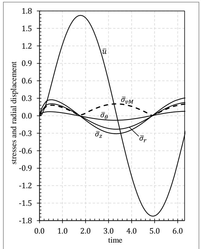
Fig. 3a. Variations of the stress components, the von Mises stress and the displacement with time at  $\bar{r} = 0.5$  based on B.C. 1 for the parameter set  $\nu = 0.3$ ,  $A = 2.0$  and  $\bar{\alpha} = 1.75$ .
