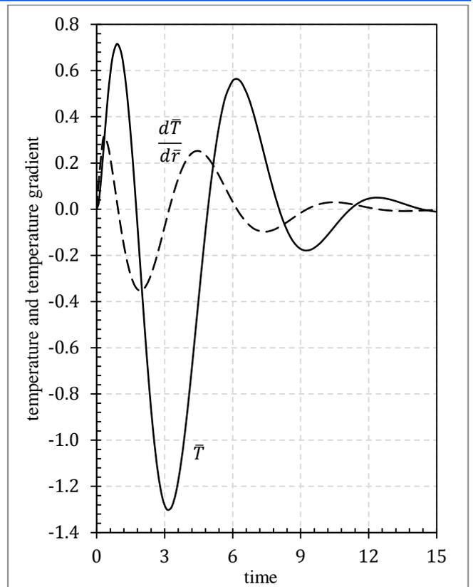
Fig. 2b. Variations of temperature and temperature gradient with time at  $\bar{r} = 0.5$  based on B.C.2 for the parameter  $\nu = 0.3$ ,  $A = 2.0$  and  $\bar{\alpha} = 1.75$ .
